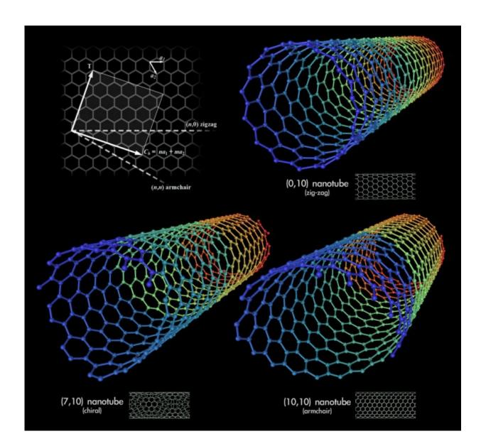
Different types of nanotubes: 1) zigzag, 2) chiral and 3) armchair (or dentated).
