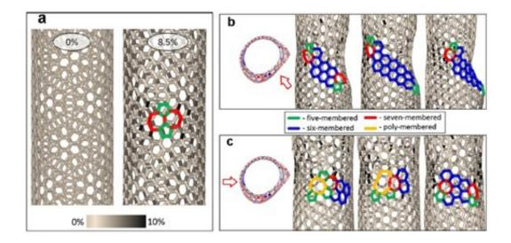
The process of the nanotube structure changing: a) stretching with the first defect formation; b) the restructuring of related carbon bonds; c) the formation of new defects and the continuation of the restructuring of links. Credit: © NUST MISIS
