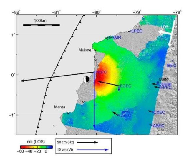
Coseismic displacement field from InSAR and GPS data after the 16 April 2016, Mw7.8 Pedernales Earthquake. Credit: Béjar-Pizarro et al., 2018
