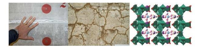
The cracks in the concrete caused by AAR form in tiny crystal fissures (middle photo) and are immediately visible to the naked eye (left-hand photo). An alkali calci-um silicate hydrate, the structure of which was clarified with Empa's help in 2016, is behind the damage (right-hand photo).
