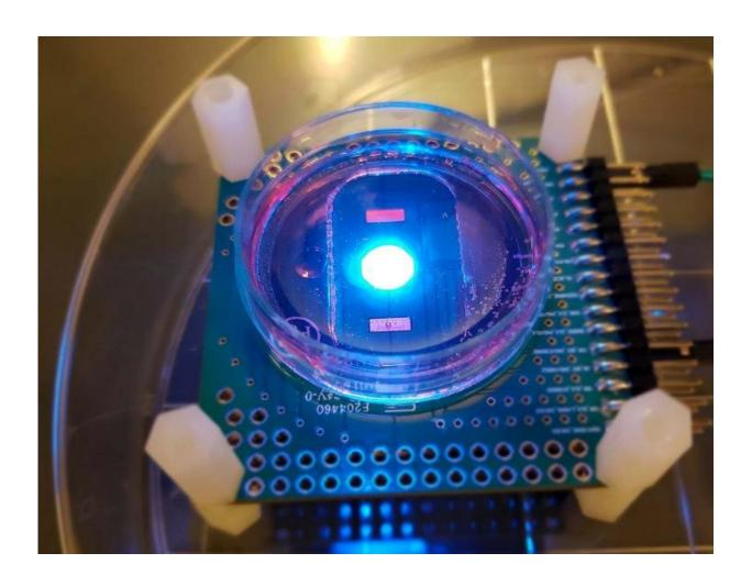
CMOS multi-modal cellular interface array chip in operation in a standard biology lab. Credit: Georgia Institute of Technology
