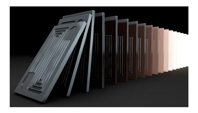
A recent development would make electricity generation from the sun's heat more efficient, by using ceramic-metal plates for heat transfer at higher temperatures and at elevated pressures. Credit: Purdue University illustration/Raymond Hassan
