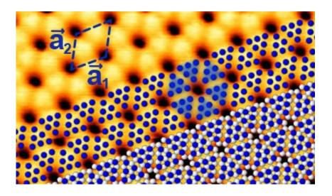
The STM image shows blue phosphorus on a gold substrate. The calculated atomic positions of the slightly elevated P atoms are shown in blue, the lower lying ones in white. Groups of six elevated P atoms appear as triangles. Credit: HZB
