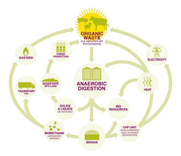
Multiple products of anaerobic digestion. Credit: Modified from ADBA with permission
