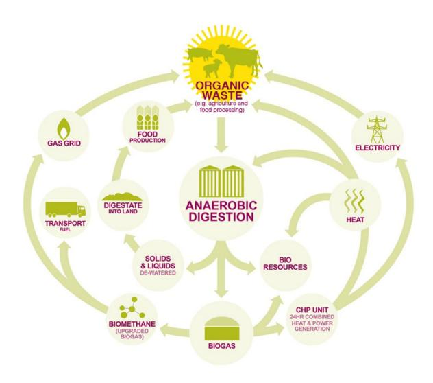
Multiple products of anaerobic digestion. Credit: Modified from ADBA with permission
