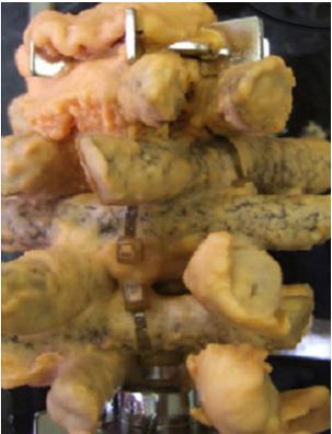
Integral to the ability of biofilm reactors to produce vitamin K are specially designed internal plastic composite supports that microorganisms adhere to and on which they build intertwined colonies -- called biofilms -- that can withstand aeration and agitation needed to spur the microorganisms to secrete more vitamin K. These photos show the supports before fermentation (top), and after, covered by biofilms. Credit: Ehsan Mahdinia/Penn State
