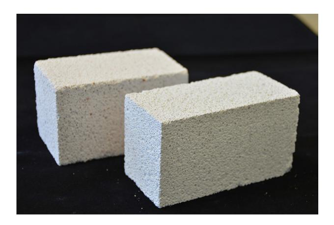
Aerated concrete made of brick (rear); aerated concrete made of sand-lime stones (front). Credit: Fraunhofer IBP
