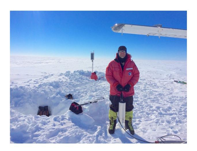
Study co-author Rick Aster during a station installation trip on the Ross Ice Shelf, holding a broadband seismometer. These sensitive sensors were buried at depths of two meters (6 feet) to record micro-scale seismic motions of the ice shelf in three dimensions over the course of two years. Credit: Rick Aster.
