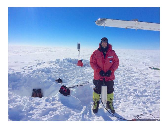
Study co-author Rick Aster during a station installation trip on the Ross Ice Shelf, holding a broadband seismometer. These sensitive sensors were buried at depths of two meters (6 feet) to record micro-scale seismic motions of the ice shelf in three dimensions over the course of two years. Credit: Rick Aster.
