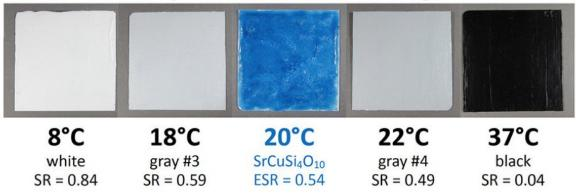
Berkeley Lab scientists measured the temperature rise above air temperature observed in full sun for five pigment-coated samples, each 75 millimeters square. The white and black samples show low and high temperatures. Credit: Berkeley Lab
