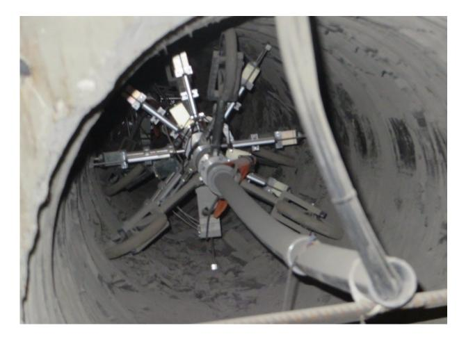
Measurement of inner displacement of the walls of a borehole for future placement of a nuclear waste package, in a French underground lab. Credit: T. Hueckel
