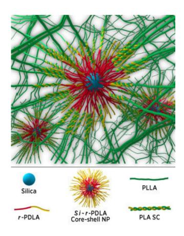
Polymeric nanocomposites comprising poly(lactic acid) with nanoparticles of silica-rubber-poly(D-lactic acid). Credit: Elsevier
