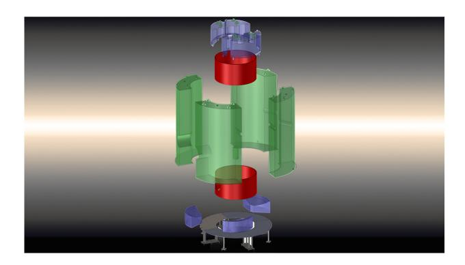
A diagram showing the components of the acrylic tanks veto system for the LUX-ZEPLIN experiment. The green and blue objects represent the clear acrylic tanks. They will be fitted snugly together and held by a metal base. Credit: LZ Collaboration
