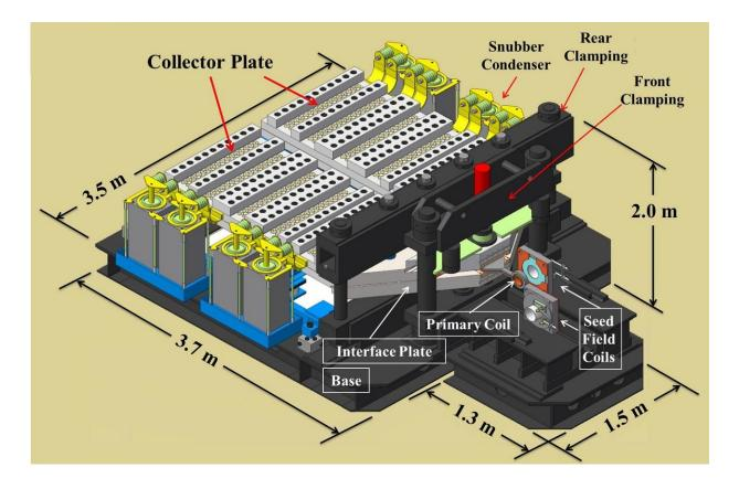
Earth's own magnetic field is 25 to 65 microteslas. The megagauss generator system creates a field of 1,200 teslas, about 20 million to 50 million times stronger. Credit: Copyright 2018 Shojiro Takeyama
