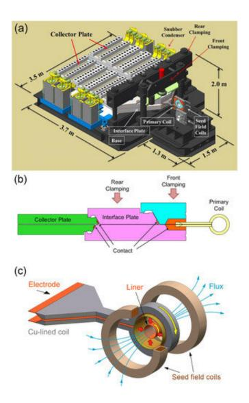
(a) Schematic view of the EMFC megagauss generator. (b) Cross section of (a).(c) Copper-lined primary coil and a pair of seed field coils. [Reproduced with permission from Nakamura et al., Rev. Sci. Instrum. 84, 044702 (2013).Copyright 2013 AIP Publishing LLC.] In (a), one of the initial seed field coils is presented in the displaced position, for more visible view of the primary coil.The primary coil is covered by an anti-explosive block made of bulk iron-steel,
