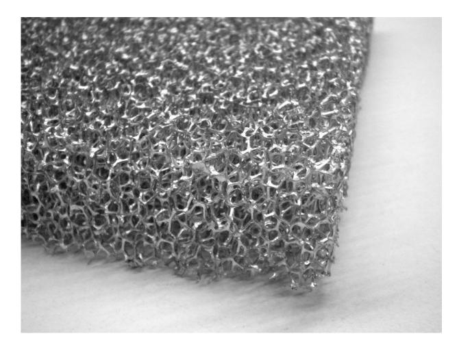
The metal sponge is manufactured in a casting process. Credit: Fraunhofer IWU
