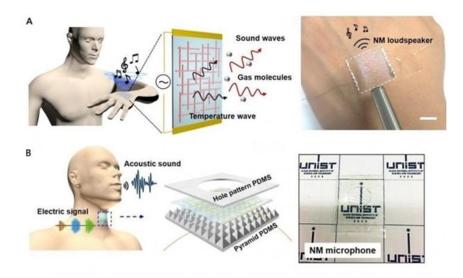
The schematic images of (A) skin-attachable NM loudspeaker with the orthogonal AgNW array and (B) wearable and transparent NM microphone. Credit: UNIST
