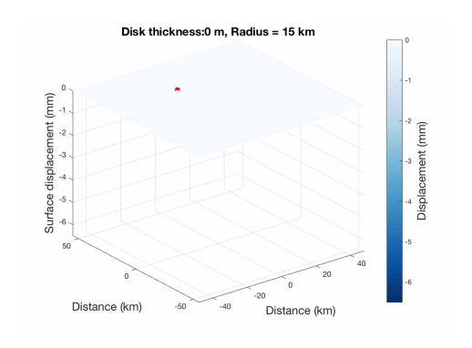
This animation shows the elastic response of Earth to increasing and decreasing a water load on the surface. The amount of depression corresponds with the expected depression the surface underwent due to the weight of Hurricane Harvey's stormwater. Credit: NASA / JPL-Caltech
