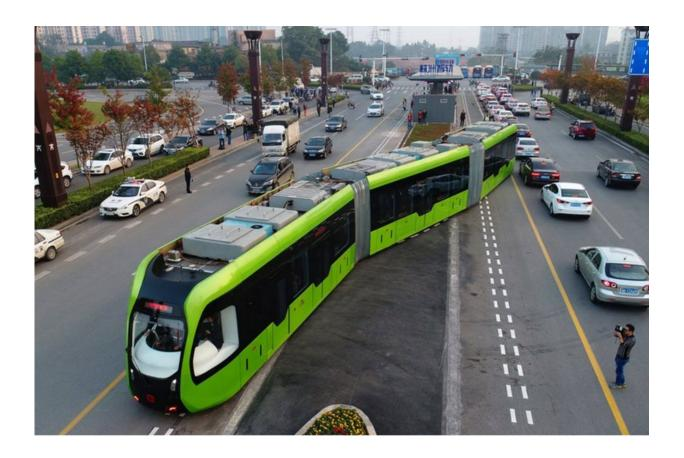
The battery-powered trackless tram, or ART, in operation in Zhuzhou, showing the trackless autonomous guidance system. Credit: CRRC Zhuzhou Institute, Author provided
