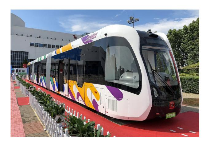
CRRC Zhuzhou Institute developed the rubber-tyred autonomous rail transit (ART) system, or trackless tram, which has already been trialled in Zhuzhou, China. Credit: Wikimedia, CC BY-SA
