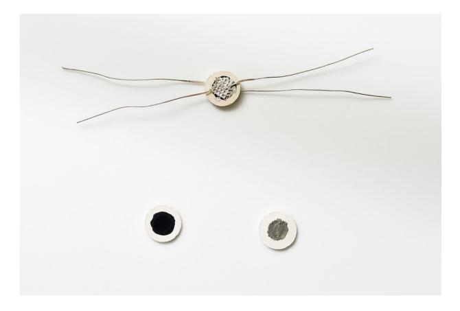
A key advance, a ceramic steam electrode that self-assembles from a woven mat, could help produce industrial hydrogen more efficiently. Credit: Idaho National Laboratory
