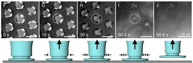
Silicone surfaces treated with plasma (below) have stronger adhesiveness than untreated surfaces (above). The material only separates from the glass surface after 50.4 seconds (I), while the untreated material already separates after 32.8 seconds (D). Credit: Emre Kizilkan
