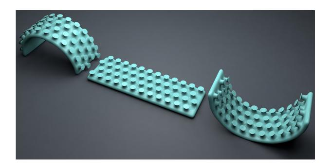
Different configurations change the adhesive effect of the silicone material, whose surface has been given a mushroom-like structure. The adhesion is best when bent concave (right). Credit: © Emre Kizilkan
