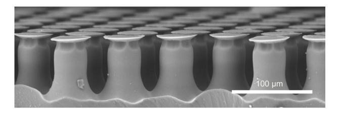
Under a scanning electron microscope, the surface of the silicon elastomer with its mushroom-like adhesive elements becomes visible. They are inspired by the microstructures on the feet of certain species of leaf beetles. Credit: Emre Kizilkan
