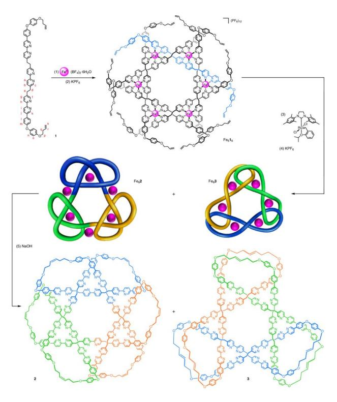
The 12 component (6 × ligand 1; 6 × Fe<sup>2+</sup>) assembly of the intermediate hexameric circular helicate  $[Fe_61_6](PF_6)_{12}$  and the synthesis of the +31#+31#+31 composite knot 2 and  $9^3_7$  link 3. Credit: *Nature Chemistry* (2018). DOI: 10.1038/s41557-018-0124-6
