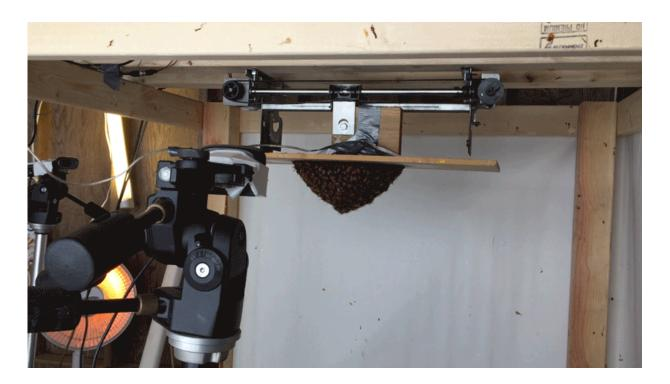
The experimental setup consists of a motor driving a wooden board, on which a cluster of honey bees form around a caged queen bee. The board can be moved in the horizontal or vertical axis at different frequencies and amplitudes. Credit: Jacob Peters, Orit Peleg/Harvard University
