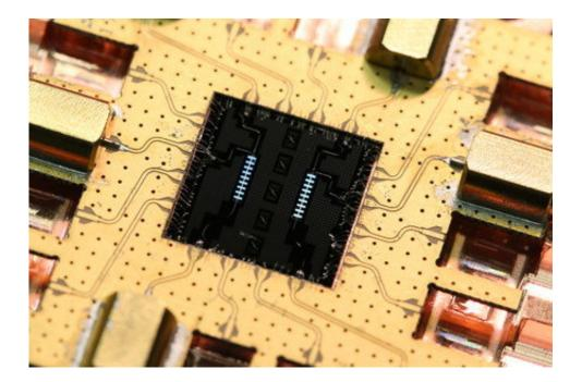
A superconducting metamaterial chip mounted into a microwave test package. The purplish-violet reflection in the center is an optical effect that can seen by the naked eye, and is the result of the diffaction of light by the periodic patterning of the microwave metamaterial. Credit: Oskar Painter/Caltech
