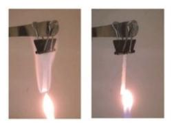
Ignition tests show how a glass fiber soaked with the promising new electrolyte (right) does not catch fire, unlike a glass fiber soaked with the conventional electrolyte (left). Credit: Environmental Molecular Sciences Laboratory
