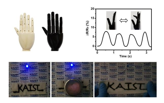
Fabrication of e-skin using various printing methods and the detection of signals for wearable and robotic applications. Credit: KAIST
