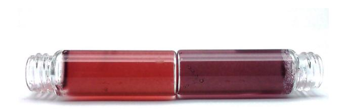
At high temperatures (left) particles move freely in the droplets and lend the material a ruby red color; they agglomerate at lower temperatures (right) and change the material's color to grey-violet. Credit: INM
