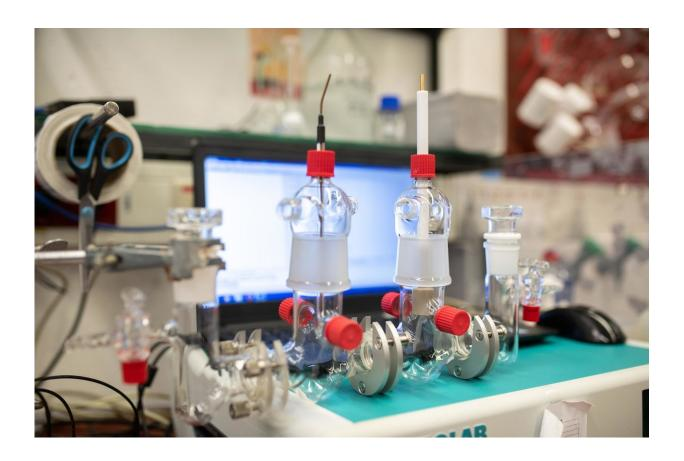
The biofuel cell tests were carried out in this electrochemical cell. Credit: Ruhr-Universitaet-Bochum
