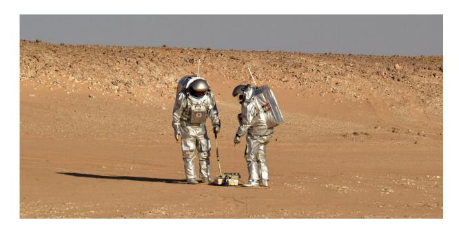
The analogue astronauts using the ScanMars radar in the Dhofar region, Oman during AMADEE-18. Credit: OEWF – Austrian Space Forum
