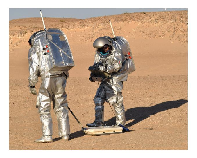
The analogue astronauts using the ScanMars radar in the Dhofar region, Oman during AMADEE-18. Credit: OEWF – Austrian Space Forum
