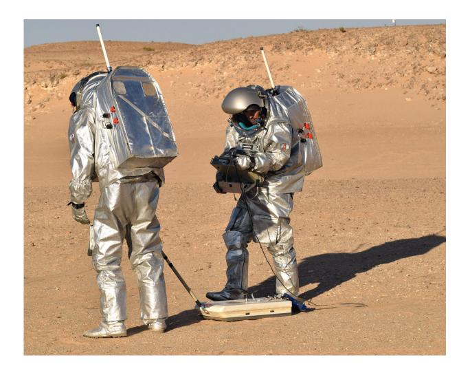
The analogue astronauts using the ScanMars radar in the Dhofar region, Oman during AMADEE-18. Credit: OEWF – Austrian Space Forum
