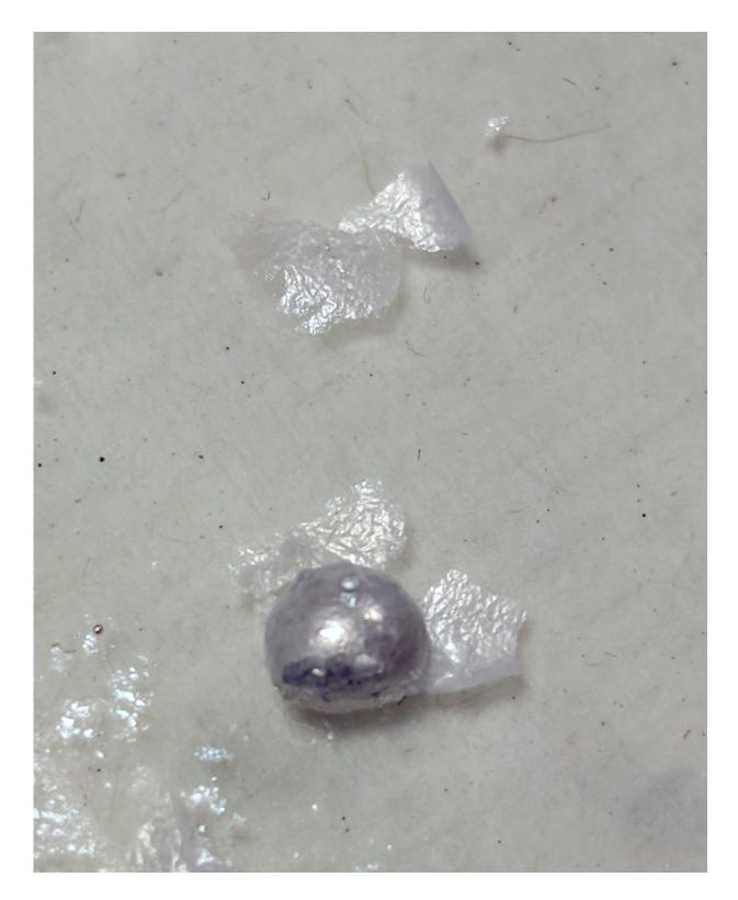
A liquid metal droplet with flakes of aluminium oxide compounds grown on its surface. Each 0.03mm flake is made up of about 20,000 nano-sheets stacked
