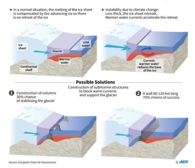
Presentation of a concept study assessing the viability of constructing massive submarine walls to slow the melting of glaciers and ice sheets and limit sea level rise.
