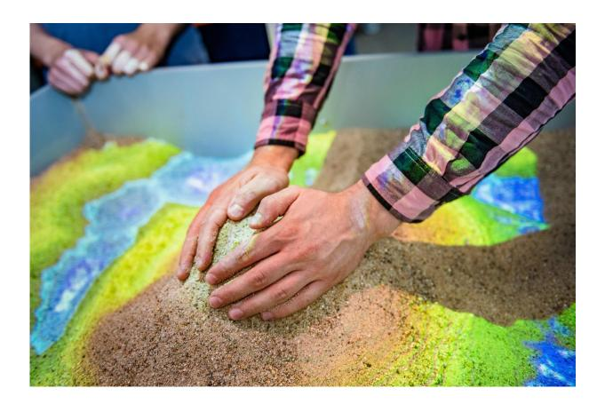
Sand is used to create an elevation profile in the laboratory. A scanner automatically detects it and projects colour-coded contour lines onto it. Virtual rain can be triggered over the sandy landscape with special hand movements. Credit: Damian Gorczany
