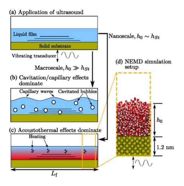
Schematics of (a) typical ultrasonic atomizer setup, (b) macroscale conjunction theory of atomization, with cavitation inside the fluid and capillary waves at the surface, (c) nanoscale acoustothermal heating and atomization, and (d) the NEMD problem setup for the simulations in this work. Credit: *Physical Review*
