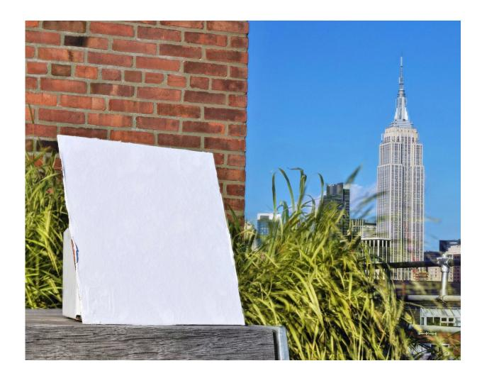
Vis version: When exposed to the sky, the porous polymer PDRC coating reflects sunlight and emits heat to attain significantly cooler temperatures than typical building materials or even the ambient air. Credit: Jyotirmoy Mandal/Columbia Engineering
