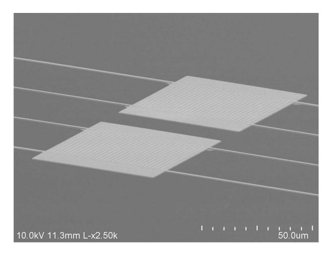
An electron microscope image of the experimental set-up with two plates, each  $0.06 \ge 0.08$  mm. At their thinnest, with a thickness of just 0.00027 mm, the heat flow between them was 100 times higher than expected. Credit: Dakotah Thompson, Michigan Engineering
