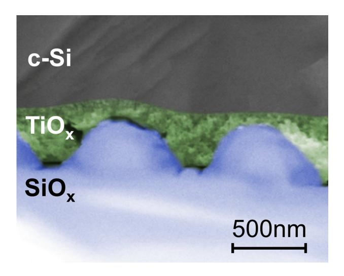
The nanostructure for capturing light is imprinted on silicon oxide (blue) and then "leveled" with titanium oxide (green). Credit: HZB
