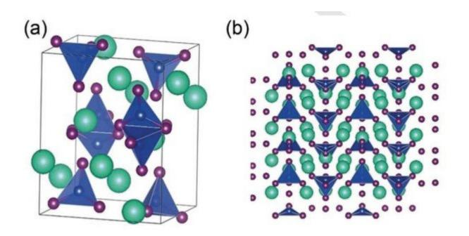
The crystalline structure of the proposed material. The green dots represent cesium atoms, and the blue bodies correspond to the  $[Cu_2I_5]^3$  units that are confined between them. The cesium atoms plus the  $[Cu_2I_5]^3$  units can be regarded as core-shell structures, which enhance the photoluminescent properties of the material. Credit: Advanced Materials
