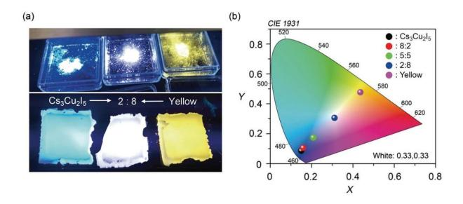
(a) By mixing the proposed material with a yellow phosphor, a white photoluminescent film was made, demonstrating one of the potential applications of this novel material. (b) The color of the produced photoluminescent film can be changed by adjusting the ratio of the proposed material to the yellow phosphor used. Credit: Advanced materials
