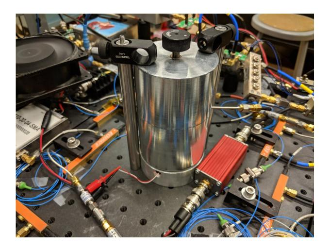
NIST's ultrafast electro-optic laser relies on this aluminum "can" to stabilize and filter the electronic signals, which bounce back and forth inside until fixedwaves emerge at the strongest frequencies and block or filter out other frequencies.
