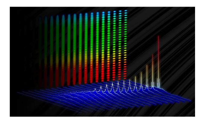
Graphic depicting how specific frequencies, or colors, of light (sharp peaks) emerge from the electronic background noise (blue) in NIST's ultrafast electro-optic laser. The vertical backdrop shows how these colors combine to create an optical frequency comb, or "ruler" for light. Credit: D. Carlson/NIST
