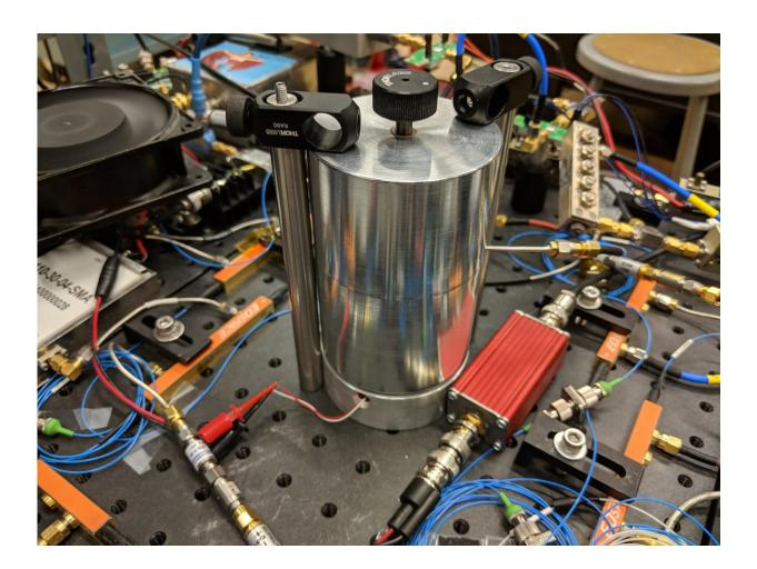
NIST's ultrafast electro-optic laser relies on this aluminum "can" to stabilize and filter the electronic signals, which bounce back and forth inside until fixed waves emerge at the strongest frequencies and block or filter out other frequencies. Credit: D. Carlson/NIST
