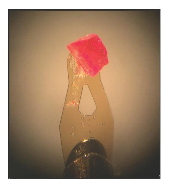
Magnified image of a superstructure built from nanoscale tetrahedral building blocks. The blocks' edges are each about nine nanometers in length. The superstructures built from them are between 200 and 300 micrometers across. Credit: Chen Lab/Brown University
