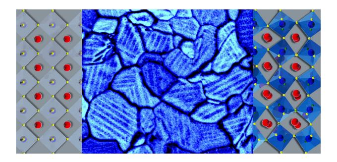
In a thin film of a solar-energy material, molecules in twin domains (modeled in left and right panels) align in opposing orientations within grain boundaries (shown by scanning electron microscopy in the center panel). Strain can change chemical segregation and may be engineered to tune photovoltaic efficiency. Credit: Stephen Jesse/Oak Ridge National Laboratory, U.S. Dept. of Energy
