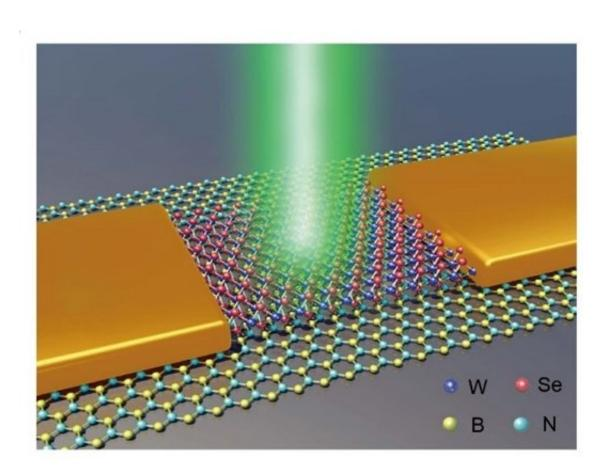
Schematic illustration of the optoelectronic memory device fabricated by layering a monolayer WSe2 on a 20-layer BN. Credit: National University of Singapore
