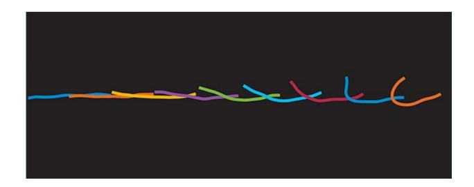
Under strong flow, the filaments bend over in a tank treading motion but remains aligned with the flow. Credit: *Proceedings of the National Academy of Sciences* (2018). DOI: 10.1073/pnas.1805399115
