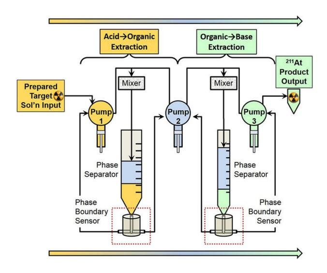
Schematic of solvent extraction module for a statine-211 (211At) isolation from dissolved bismuth cyclotron target. The process starts on the left side and proceeds to the right. Credit: Matthew O'Hara, Pacific Northwest National Laboratory
