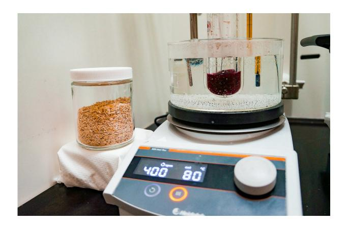
Beech wood undergoing deconstruction. Credit: Ydna Questell-Santiago (EPFL Laboratory of Sustainable and Catalytic Processing)
