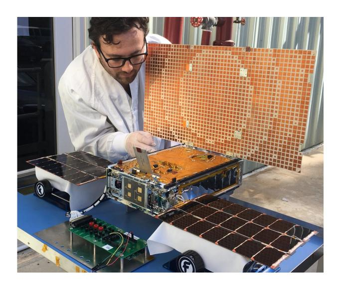
Engineer Joel Steinkraus uses sunlight to test the solar arrays on one of the Mars Cube One (MarCO) spacecraft at NASA's Jet Propulsion Laboratory. The MarCOs will be the first CubeSats -- a kind of modular, mini-satellite -- flown into deep space. They're designed to fly along behind NASA's InSight lander on its cruise to Mars. If they make the journey to Mars, they will test a relay of data
