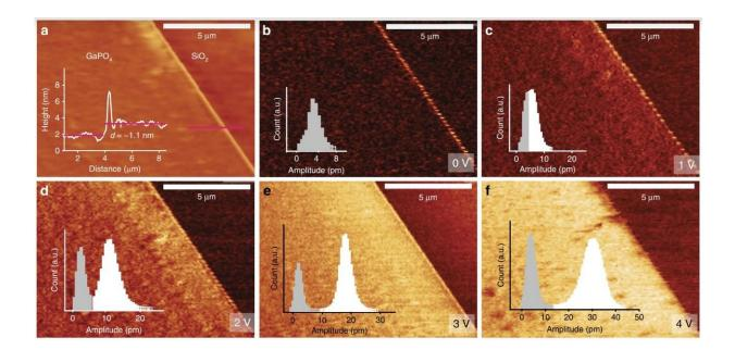
Atomic force microscopy imaging of 2D GaPO<sub>4</sub> and piezoelectric measurements at varying applied voltages Credit: FLEET
