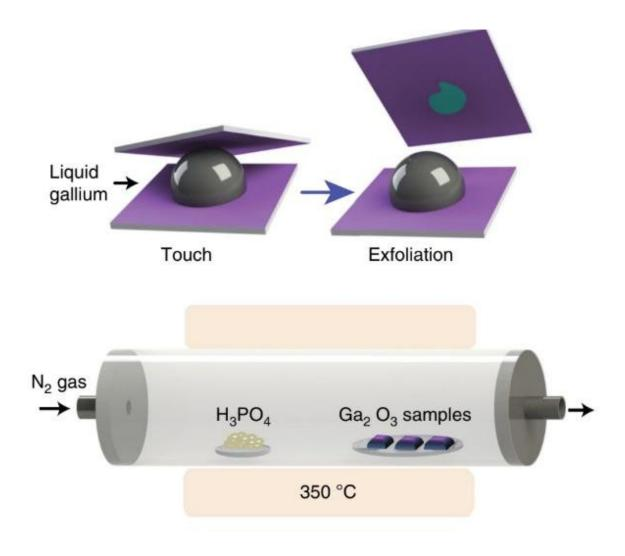
Upper: van der Waals 2D printing of Ga<sub>2</sub>O<sub>3</sub> nanosheet from liquid metal
