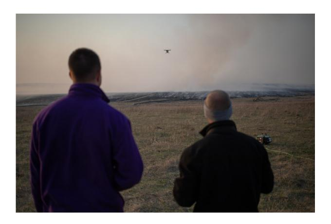
Two Kansas State University pilots fly an unmanned aircraft over a tallgrass prairie prescribed burn to gather smoke emissions data. The pilots are part of a large collaborative project that is using unmanned aircraft to improve the Kansas Flint Hills Smoke Management Plan and determine smoke constituents. Credit: David Burchfield, Kansas State University
