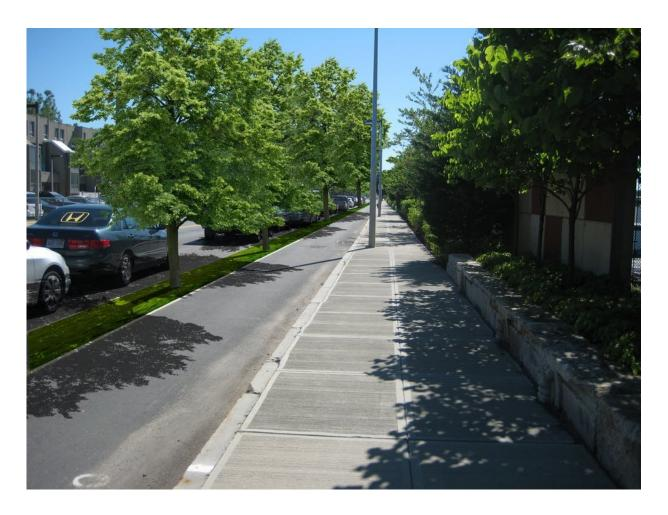
Photomontage of Western Avenue in Allston, Massachusetts, with trees separating the cycle track from the street and curb separating cycle track from sidewalk. Credit: Anne Lusk, <u>CC BY-ND</u>
