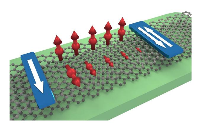
Illustration of anisotropic spin transport in a bilayer graphene flake between injector and detector electrodes. The out-of-plane spins are well transmitted whereas the in-plane spins decay fast. Credit: Talieh Ghiasi / Van Wees Lab / University of Groningen
