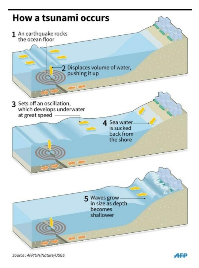
Factfile on how a tsunami occurs. 90 x 122 mmFactfile on how a tsunami
